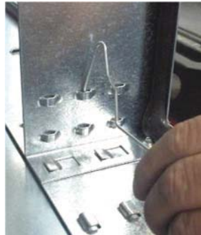
Figure 86: Insertation of the clips
