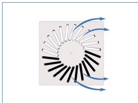
Setting of the air control blades
